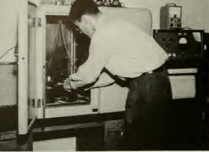
Measurement of Bacterial Growth by Constant Nephelometer (Dairy Research Laboratory)
